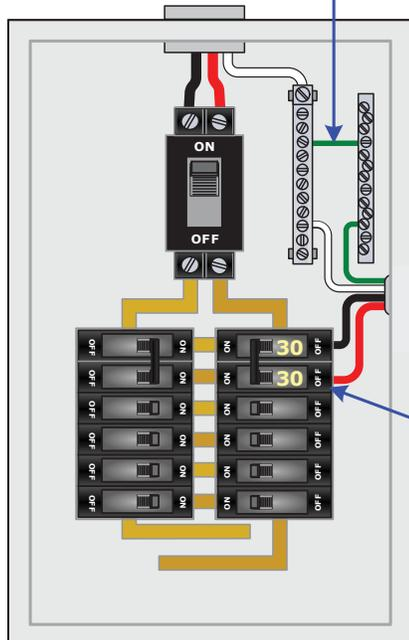
Maximum 30-amp breaker (double pole) required to inverter AC input
