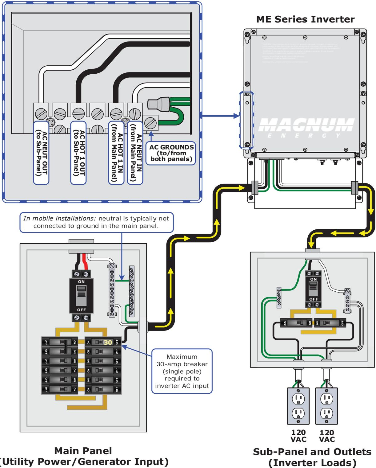
Figure 2-10, AC Wiring for Single In – Single Out (30A) Configurations
