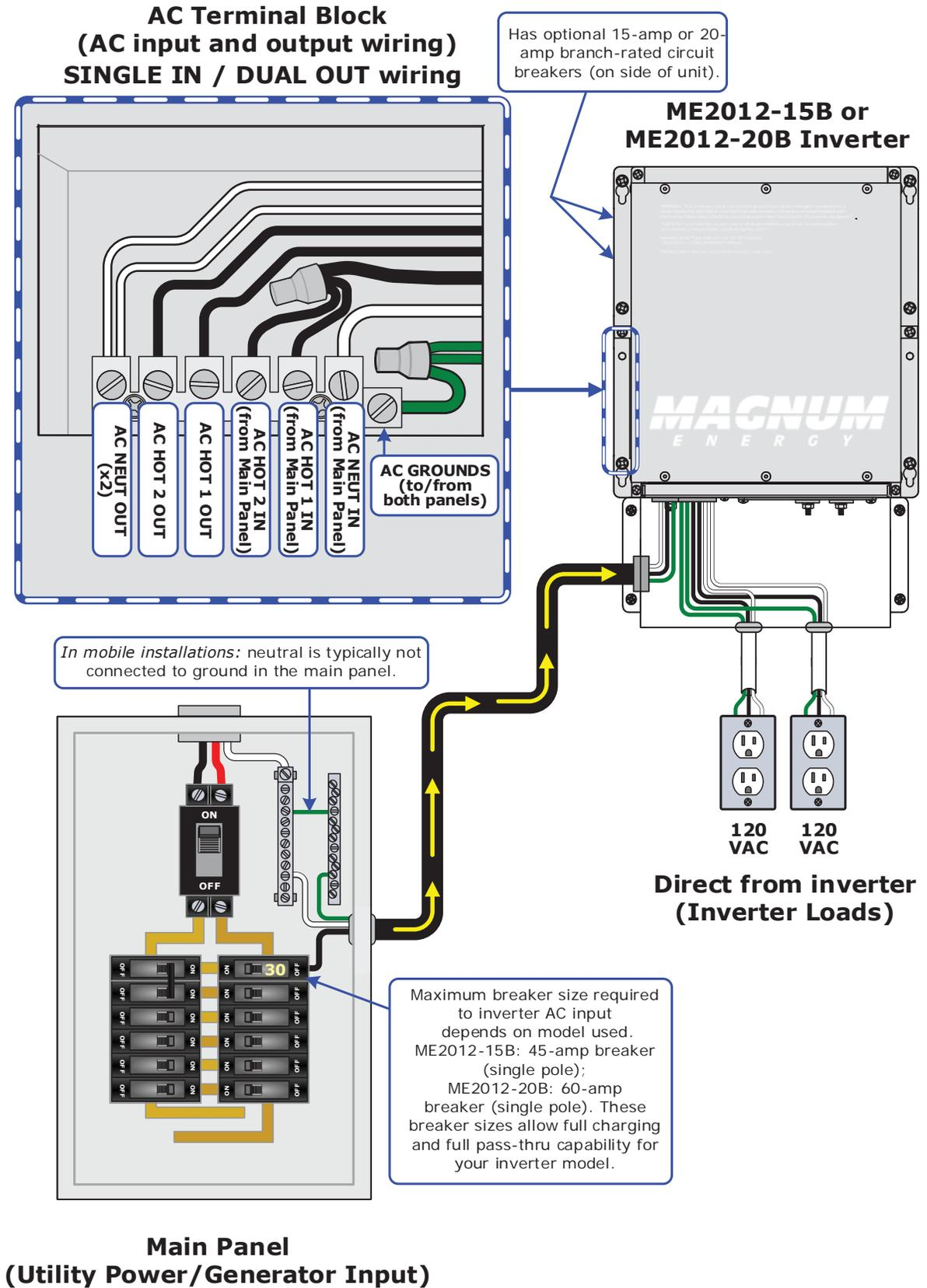
Figure 2-12, AC Wiring for Single In – Dual Out Configurations
