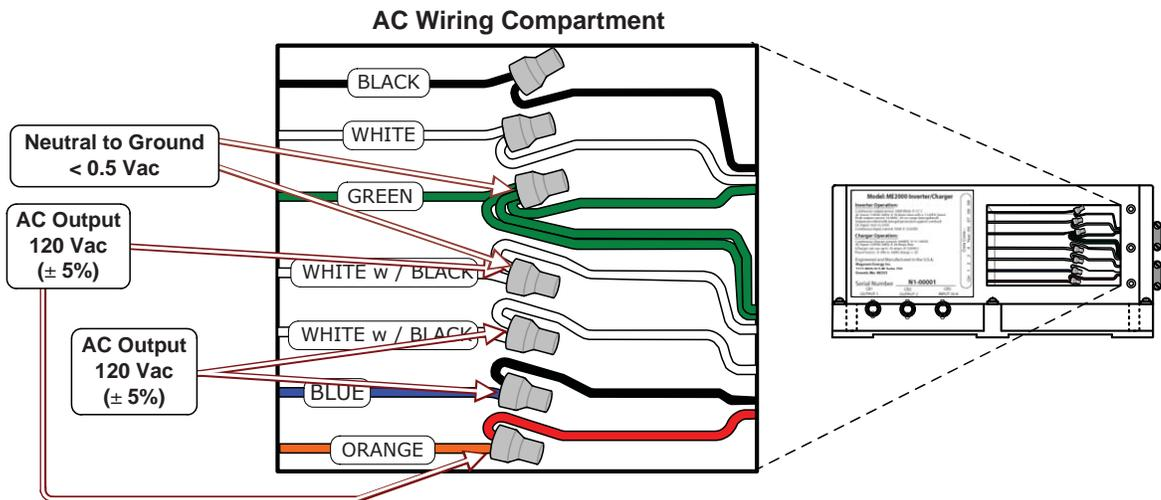
Figure 2-23, AC Voltage Checks (ME2000-15B/-20B models)
