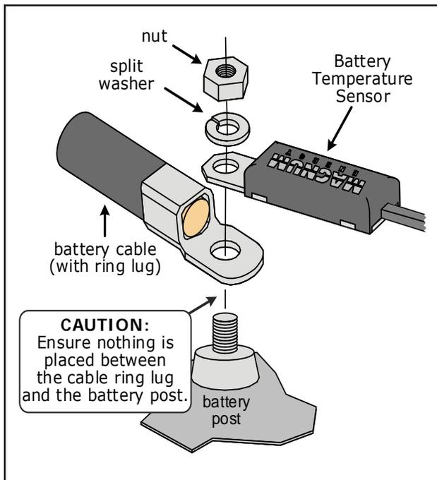
Figure 2-6, Battery Hardware Installation
