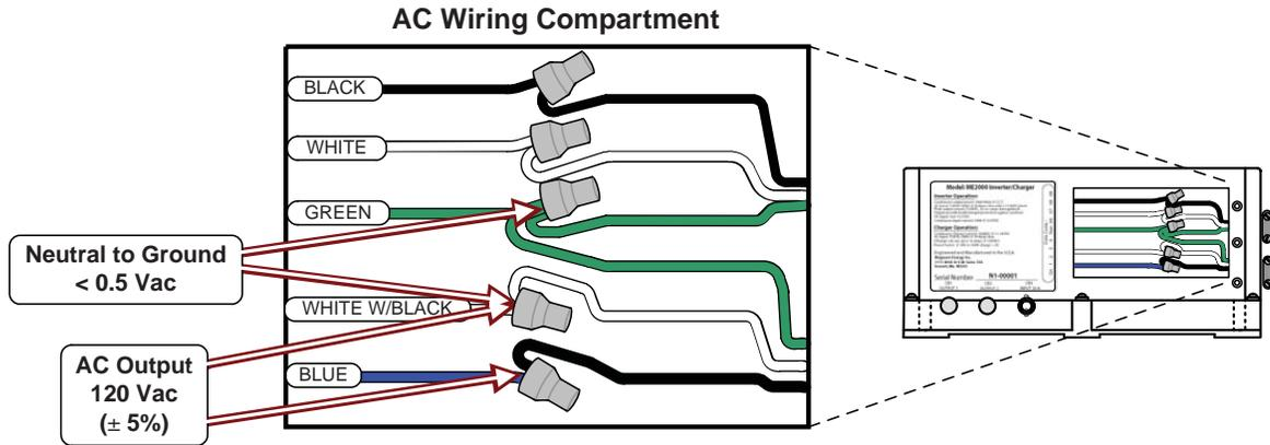
Figure 2-22, AC Voltage Checks (ME2000 model)
