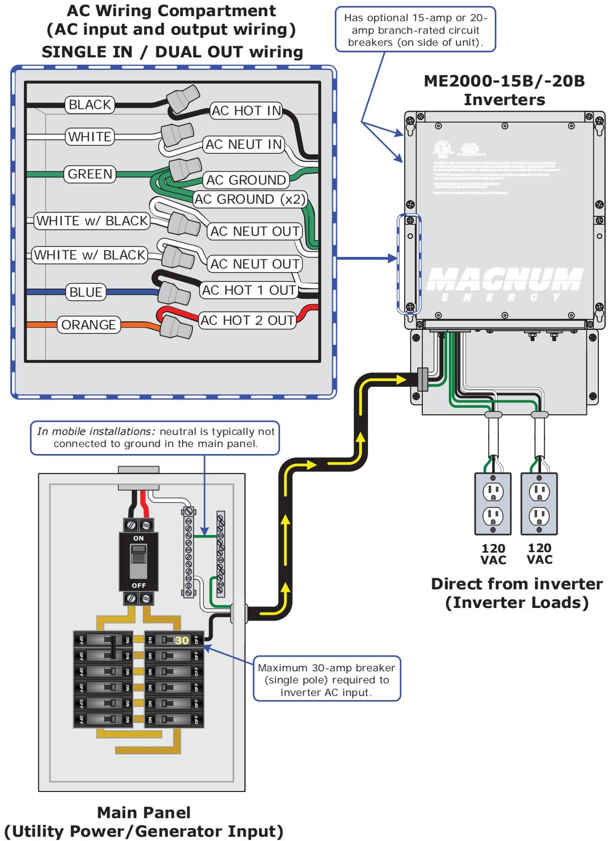
Figure 2-16, AC Wiring for ME2000-15B/-20B Models
