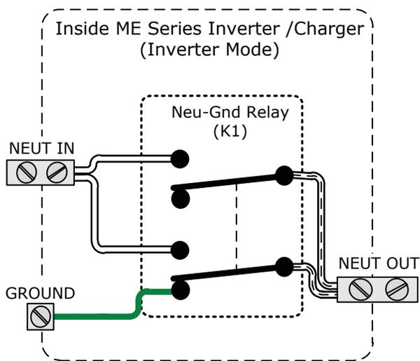
**Figure 2-17, Neutral-to-Ground Connection (Inverter Mode)**
