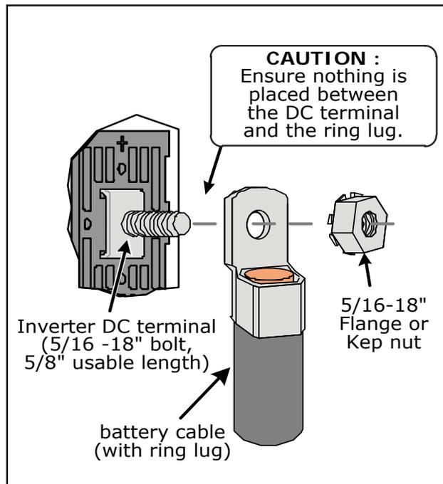
Figure 2-7, Inverter DC Hardware Installation
