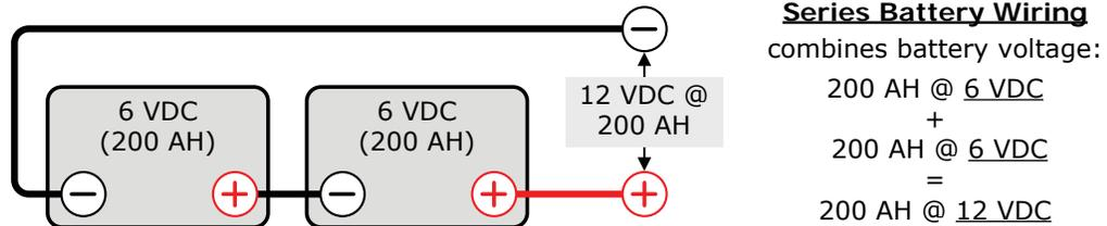
Figure B-1, Series Battery Wiring
