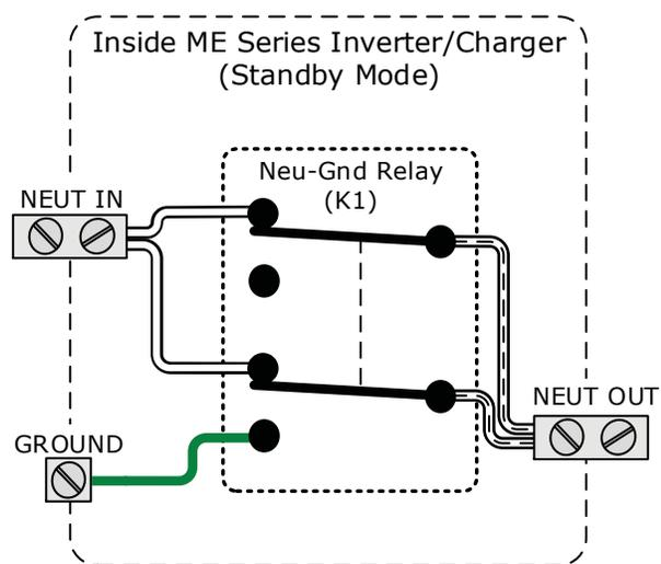
**Figure 2-18, Neutral-to-Ground Connection (Standby Mode)**
