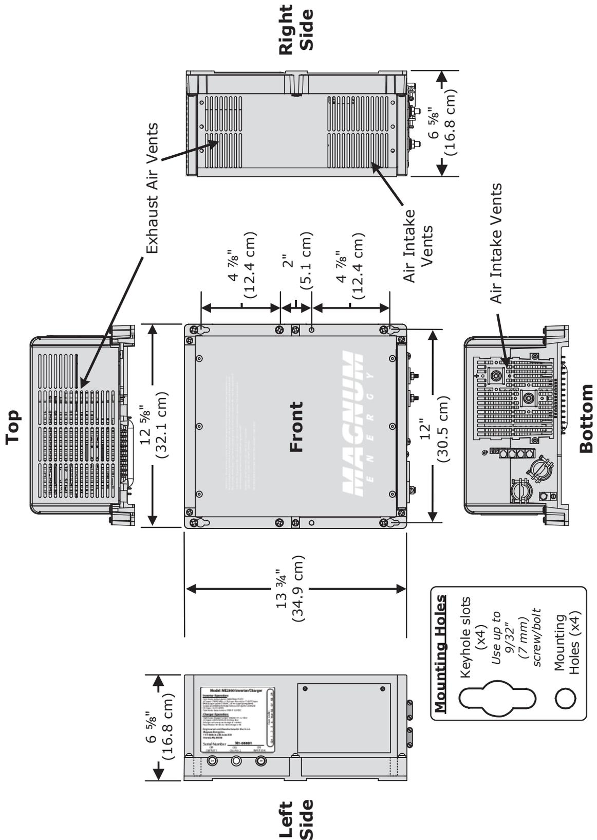
Figure 2-4, ME2000 Series Dimensions and Side Reference
