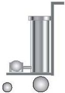
Many Heat Treating facilities utilize portable filter systems to clean the oil in the furnace sumps. There are advantages to using this off-line method for filtration. These systems can run when the Heat Treat machines are off. Often, these systems are more robust than the systems on the Heat Treat Machines.
