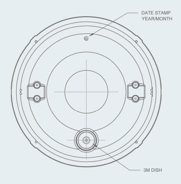
**3M™ iD Markers** are designed to provide an accurate, convenient, long-lasting method of marking underground assets. In addition, these markers may be programmed to include customer specific information such as facility data, type of application, material type and size, placement date and other important details.
