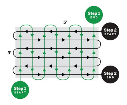
If the floor is in good condition (without visible scratches), you may only need to use the Hone and Satin pads for polishing.
