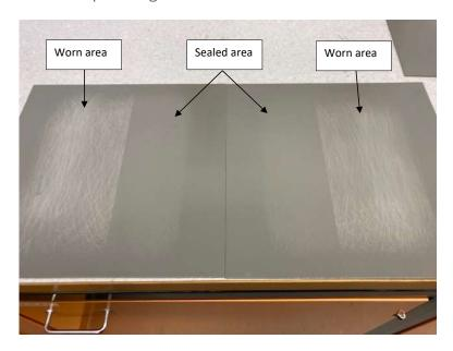
**Quartz Composition Tile after dirt pickup test;** before cleaning:
