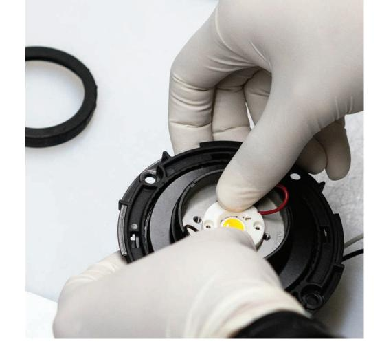
As needs change, light should flex to meet them. Unlike other warm dimming products, DMF's Warm Dim doesn't rely on discrete LEDs or complicated control systems. Our modules are powered by one premium COB chip that utilizes color mixing phosphors to produce a relaxing glow as it dims while maintaining DMF's trademark quality and ease-of-use. Impressively, it accomplishes all this from the control a single standard dimming switch.
