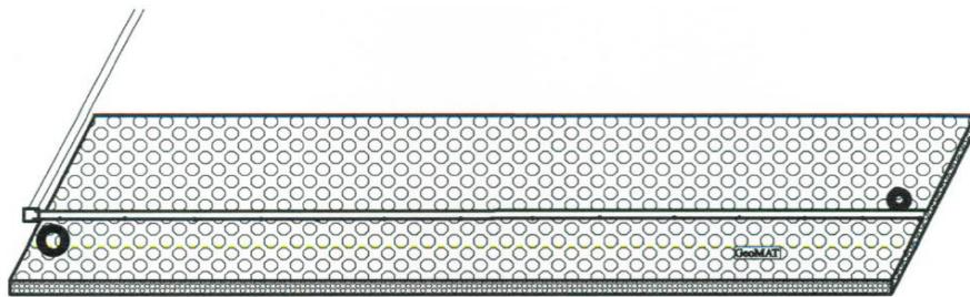
Hole spacing is every 12", 1/2" hole at 4 & 8 O'clock, starting 4 O'clock 6" from end and 8 O'clock Holes at 12" from end.
