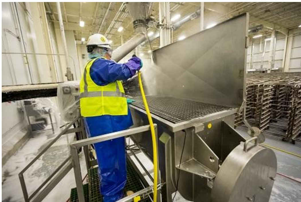
A sanitation worker applies a pressure hose to bakery equipment as part of the cleaning process. Equipment designed for easier cleaning can speed the process considerably. Photo: Packers Sanitation Services Inc.
