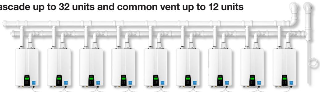
With Navien cascading technology, when a unit gets up to 80% capacity the next unit will turn on to help meet requirements. This demand ratio will continue until all 32 units are generating hot water. The Navien cascading system also balances out the workload of each unit for longer life. Building penetrations are reduced with Navien's common venting feature.
