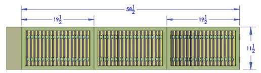
The PCP Compound is comprised of PCP Standards. As with the Compounds, the Standard's first dimension is the measurement of the panel across the lamps; the second measurement is along the lamps.
