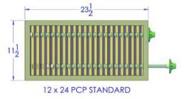
All PCP Compound units are 6" deep nominal; actual dimension is 5 13/16". The catalyst is pleated at one pleat per inch. The lamps are spaced 6" from each other on all models, then centered over the width of the panel. The ballast tray is incorporated into the unit to house the
