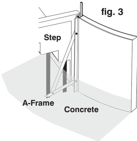
**NOTE:** Complete backfill is required around the step.
