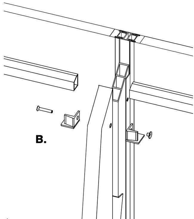
**Bracing kit will include a longer capscrew where braces are used on two adjacent straight panels.**
